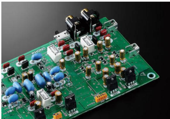
The phono amp is comprised of an MC head amp and an equaliser amp, each of which are discretely configured, resulting in a rich sound with pronounced musicality, when playing vinyl records with both MC and MM phono cartridges.
